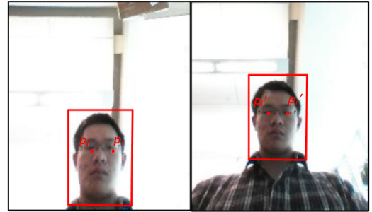
Figure 12: Prediction window generation based on eye feature points mapping.
