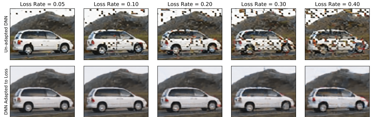
Figure 11: Visual quality comparison of DNN before (top) and after (bottom) adaption to packet loss. Both models are trained with MS-SSIM loss. DNN with adaption is trained with packet loss rate of 0.1. Adapted DNN could mask reconstruction errors due to packet loss and its image quality degrades more gracefully, even if the actual loss rate deviates from the trained rate.
